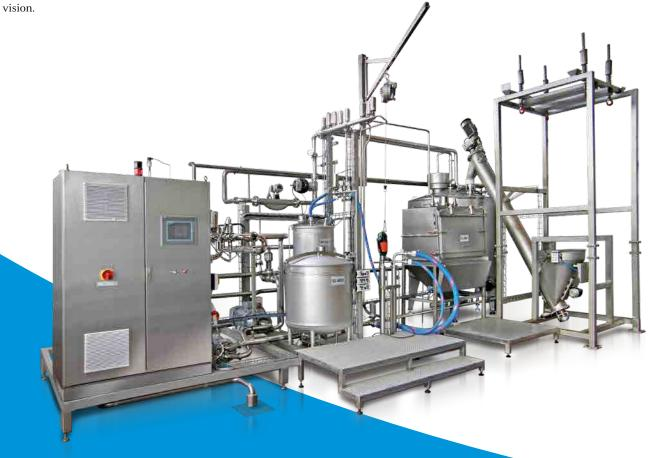
Modular batch mixing systems provide a user-friendly, high performance, intelligent and flexible production solution for a wide range of recipes
